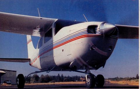
stabilizer and wingtip extensions, and they also managed to shed the heavy pitch downspring and bobweight. In the landing flare, it's possible to make very delicate pitch adjustments in the R where as in, say, the N model, it's more a vank-and-watch affair.
